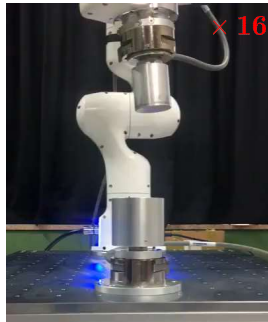
• Peg-in-hole experiment using PANDA manipulator
