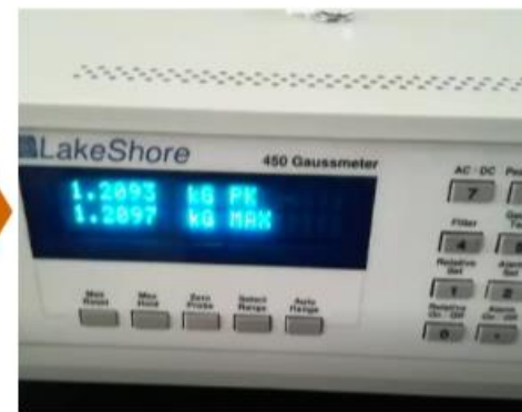
Strength of UPEMF shown in Gaussmeter
